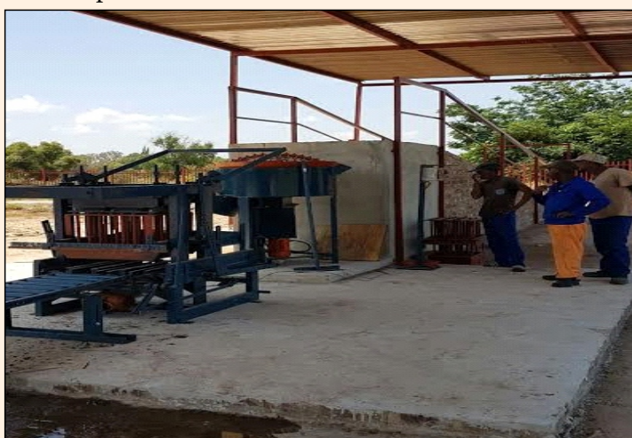
CHRISTIANA BRICKMAKING PLANT: 10 temporary local jobs were created. The plant can produce up to 5 000 bricks per shift and double the amount in two shifts. A maximum of 40 EPWP work opportunities can be created. EPWP Beneficiary to be trained as brick making; Brick Paving and Business Skills. Cooperatives on Brickmaking and Brick paving to be developed.
